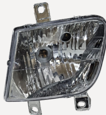
Head Lamp Assembly Plastic Lens Consisting of Driving and Passing Beam
